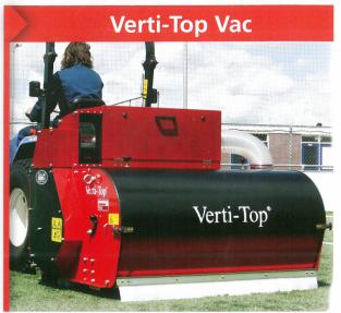
The Verti-Top Vac is a cleaning machine, in which a vacuum cleaning mechanism has been incorporated. While the vibrating mechanism is collecting the larger debris partials, the vacuum system removes the fine material, such as dust, hair and the like into a washable filter bag.
