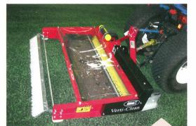
The PTO driven version of the Verti-Clean makes it easier to remove larger amounts of dirt, litter and debris as the rotary speed of the brush can be varied.
