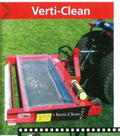
The Verti-Clean picks up surface debris with a rotating brush, which throws it on a vibrating sieve. The sieve filters infill material back on to the playing surface, while retaining the debris. Both the rotating brush and the vibrating sieve are powered by the movement of the machine.
