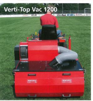
The Tow Behind Verti-Top Vac utilises the same innovative cleaning technology as the tractor mount version by quickly and effectively removing debris from the surface while gently brushing and grooming the turf fibres. All material that is brought up is sifted out on a vibrating shaker screen with the clean infill being returned to the turf and the debris sifted into two easy-to-empty bins.
